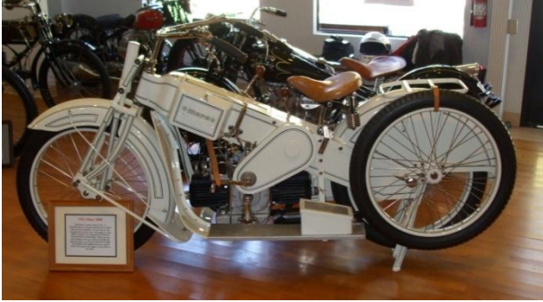
1921 Mars. 8 hp from 1000 cc. twin designed by Maybach (!). Note spare. Note 2 chains, one to a low final drive sprocket, the other to a high final drive sprocket.
