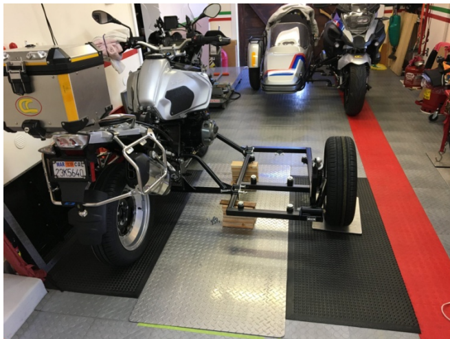
Test fitting of sidecar frame.
