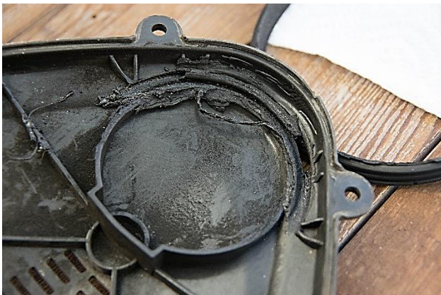
Damage to the front engine cover.
