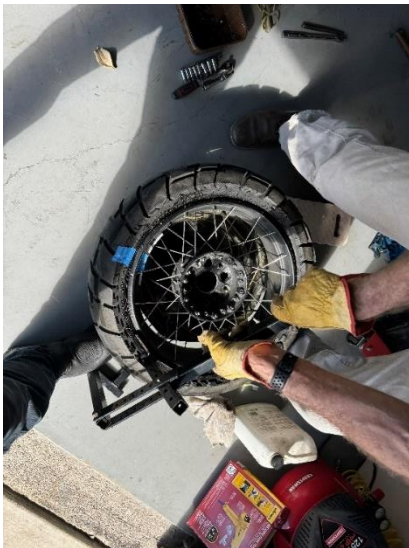
6. Mark the tire and rim location to match later for maintaining tire balance.
